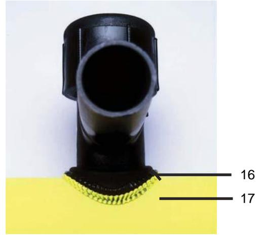
16. Proper alignment, force and melt
