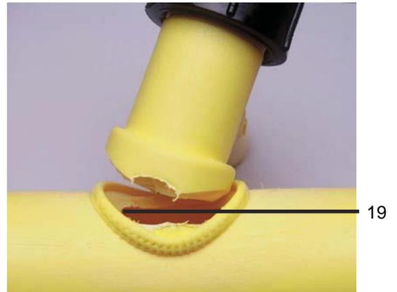
19. Material pulled from pipe when impact tested
