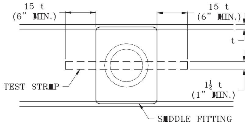
6. Visually inspect the joint for any voids, gaps, misalignment or surfaces that have not been properly bonded.
