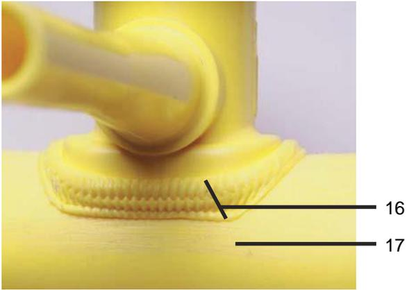
16. Proper alignment, force and melt
