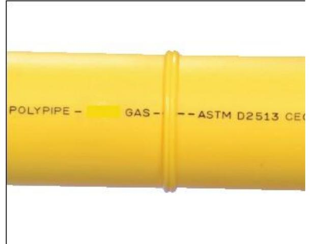
Proper alignment and double roll-back bead.
