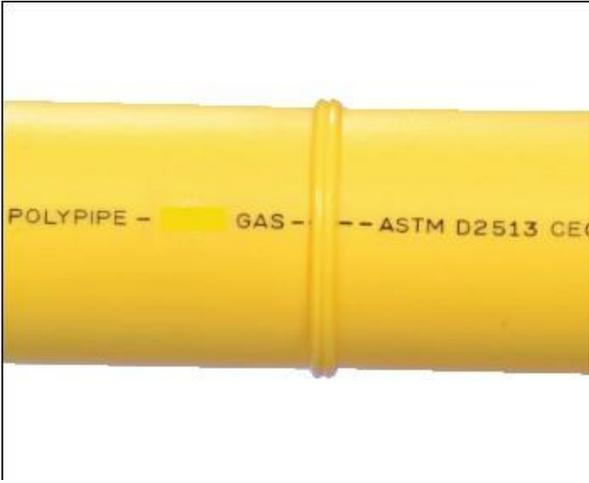
Proper alignment and double roll-back bead.
