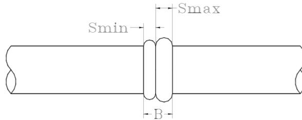
**NOTE:** When butt fusing to molded fittings, the fitting side bead may have an irregular appearance. This is acceptable provided the pipe side bead is correct.
