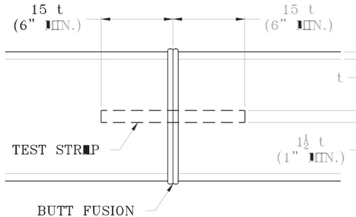
6. Visually inspect the cut joint for any indications of voids, gaps, misalignment or surfaces that have not been properly bonded.
