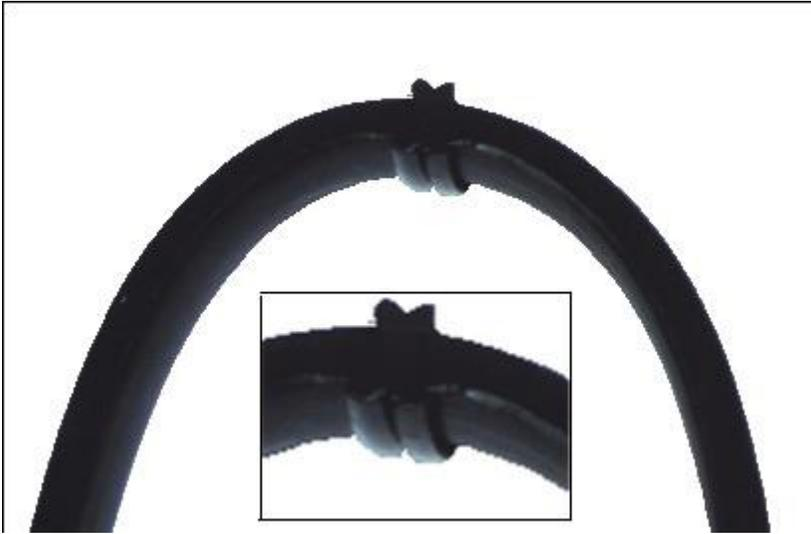
Bend back testing. No gaps or voids. (See Figure I)
