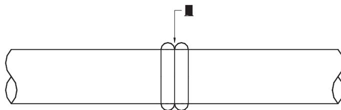
2. The displacement (V) between the fused ends must not exceed 10% of the pipe/fitting minimum wall thickness.
